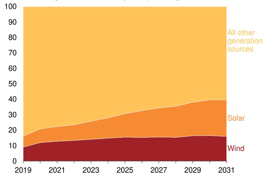
Notes: Based on AEMO's Integrated System Plan neutral scenario. Solar includes both large-scale and rooftop solar.
